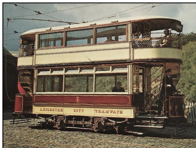
1017's original truck under restored Leicester tram 76 at Crich Museum seeming unchanged.
